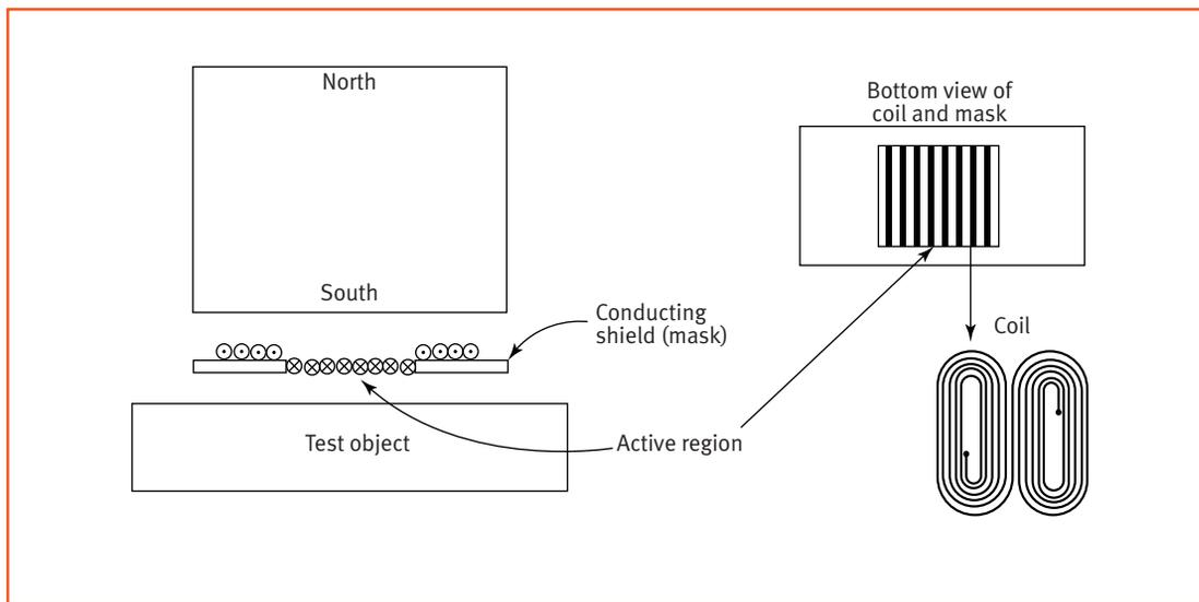
Figure 3. A normal beam shear wave EMAT (not to scale).
