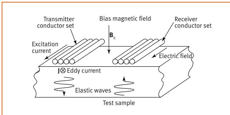
**Figure 1. Representation of a general Lorentz force EMAT consisting of transmitter and receiver conductor sets placed in a bias magnetic field near a metallic test sample (adapted from Maxfield and Wang 2018 with permission).**
