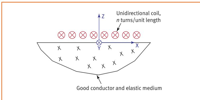
**Figure 2. Unidirectional coil above bulk metal surface.**
