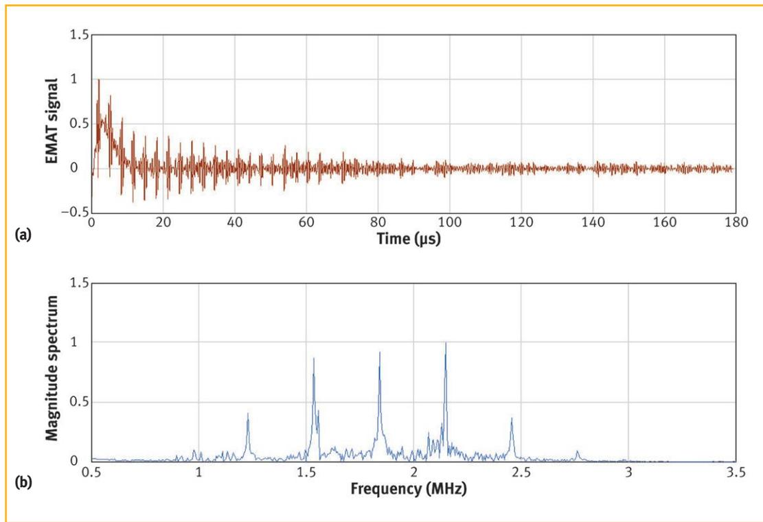
**Figure 7. Normalized normal beam shear wave signal obtained on a 5.29 mm steel plate: (a) normal beam shear wave signal; and (b) fast fourier transform of normal beam shear wave signal.**
