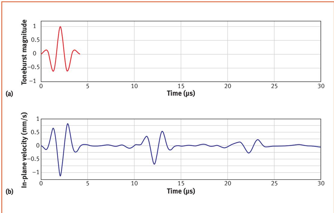
Figure 5. Waveforms of the excitation current flowing through the coil and the calculated particle velocity at the upper surface of the test object: (a) the toneburst excitation used in simulation (normalized); and (b) the calculated in-plane particle velocity under the center of the transmitter.
