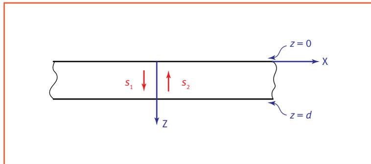
Figure 6. Normal beam shear waves ( $S_1$  and  $S_2$ ) traveling in upward and downward directions.
