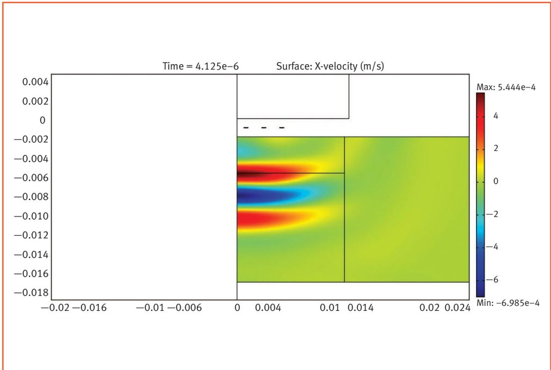
Figure 4. In-plane particle velocity (in X-direction) in the cross section of the test object.
